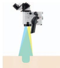
At low magnification, the illuminated field (yellow) fills in the field of view (green) completely.
