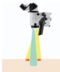
In conventional microscopes, as magnification increases, the field of view decreases. The illuminated field remains unchanged. Light outside the field of view (red) could potentially cause tissue burns.
