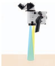
AutoIris™ automatically decreases the field of illumination as the field of view gets smaller. There is no peripheral illumination to cause tissue burns outside the field of view.
