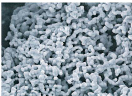
**AgPROTECT™:** Typical structure of a metal powder (Ag) created by inert gas condensation (nanopowder). This antimicrobial nano silver coating reduces infectious agents on the instrument and their transmission to users.
